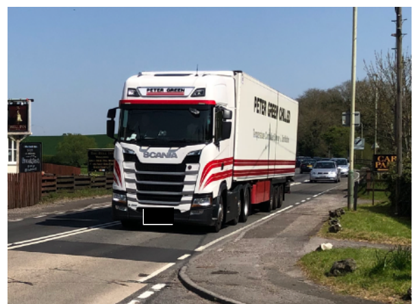
Figure 6: Peter Green Chilled HGV registered after 1 Sep 2016 - corner lights but no high level lights (LHS). Newer HGV registered after 1 Sep 2018 with high-level running lights in addition to high level corner lights.
